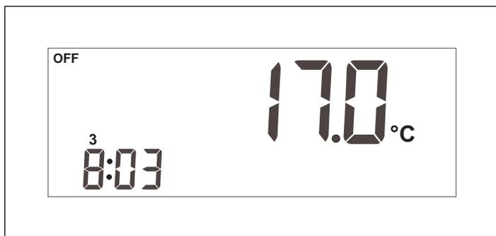
Entering this mode gives access to the configuration values that could have been changed temporarily, the set points and fan status.
